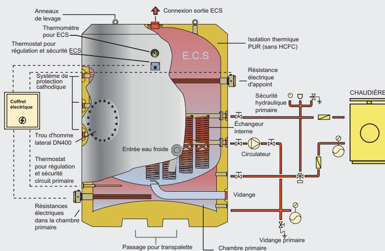
MODÈLES MVV-1500...4000/ESB. INSTALLATION COMBINÉE "CHAUDIÈRE / ÉLECTRIQUE"
