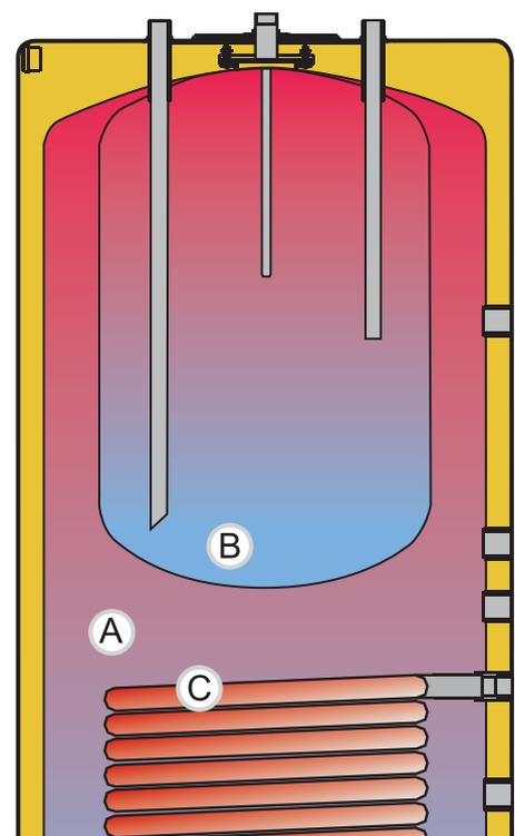
(A) BALLON D'INERTIE, (B) BALLON ECS, (C) SERPENTIN SOLAIRE
